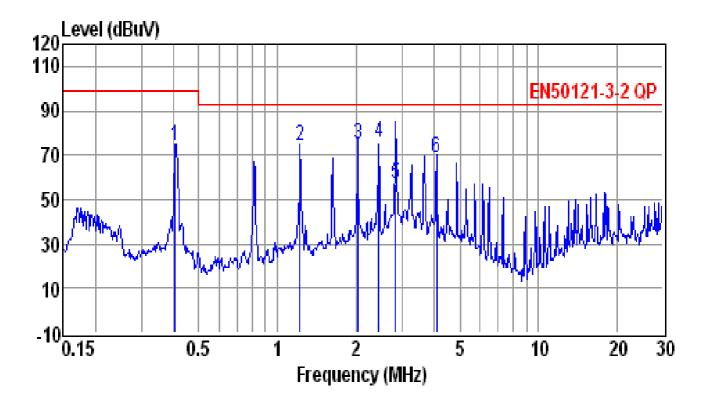
Site : conducted #1 Date : 12-17-2013 Condition : EN50121-3-2 QP LISN : NEUTRAL Tem / Hum : 23 °C / 52% Test Mode : Operation Mode
